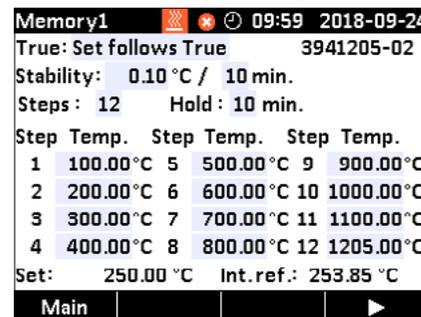
In AUTOSTEP mode you can program as much as 12 temperature steps and at the same time set the dwell time. Even the stability criteria can be programmed. Just start the sequence and the calibrator will run through the steps.
