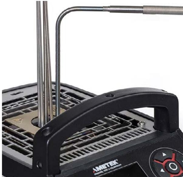
Insert heat loss due to mass loading from multiple or large sensors can be a challenge for most dry-block calibrators. The CTCs advanced feedback algorithms combined with the external reference sensor effectively addresses these challenges and makes the accuracy even better.
