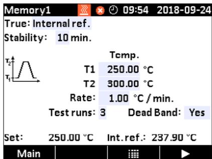
Switch test calibration is a perfect time saver. Start the switch calibration and come back to note the results after the test. You decide if you want the deadband or not - and the test can be repeated automatically in up to three subsequent runs.
