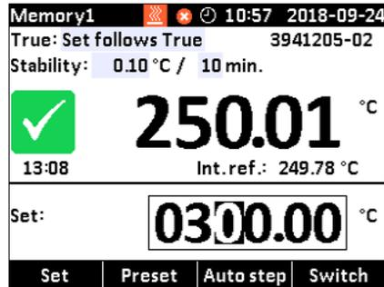
The fastest and simplest way of starting the calibrator. Simply press SET and type in the wanted temperature and off you go.
