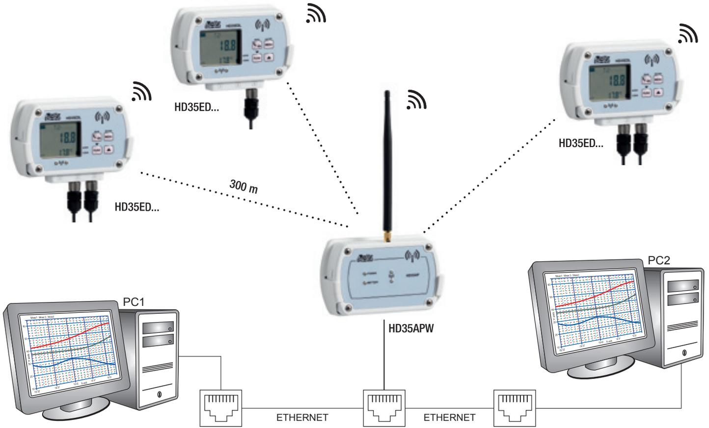
**System with connection between PC and base unit via Wi-Fi local network**
