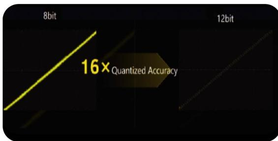
**12-bit** vertical resolution provides 4096 vertical digitizing levels
