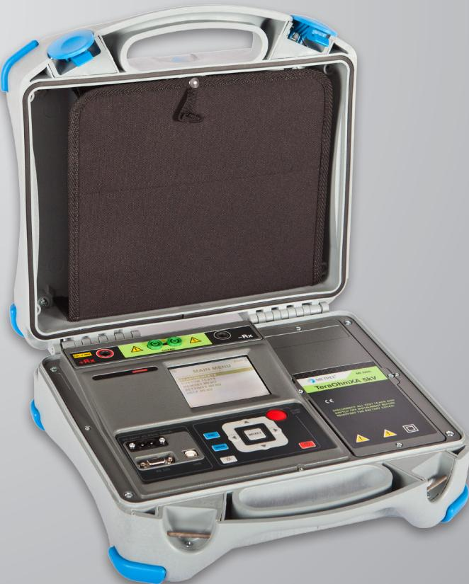
MI 3205 TeraOhm XA 5kV is a portable battery (Li-ion) or mains powered test instrument with excellent IP protection (IP65 case closed and IP54 case open), intended for diagnosing of Insulation Resistance by using high test voltages of up to 5 kV. It is designed and produced with the extensive knowledge and experience acquired through many years of working in this field.
