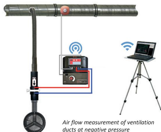
*Air flow measurement of ventilation ducts at negative pressure*
