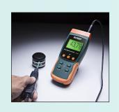
Extech's SDL900 measures and datalogs both AC and DC Magnetic Field in Gauss and mT (milli Tesla) with a uniaxial Hall effect sensor and built-in ATC. Internal memory stores up to 99 readings, while SD memory card (included) allows continuous datalogging and readings can easily be exported to an Excel® format for further analysis.
