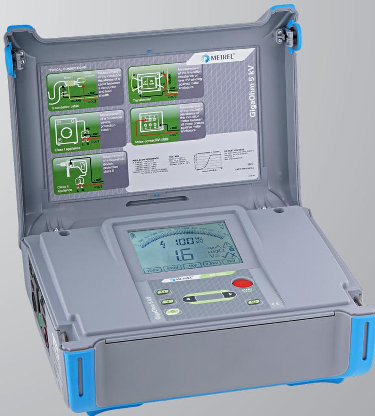
The MI 3202 GigaOhm 5 kV provides quick and accurate testing of insulation resistance. Five test voltages up to 5 kV and 1 T $\Omega$  resistance measuring range cover most of the industrial and power distribution applications. The large analogue / digital LCD screen with backlight offers easy reading of test results. The instrument is placed in a rugged carrying case which allows to use it in harsh environments.
